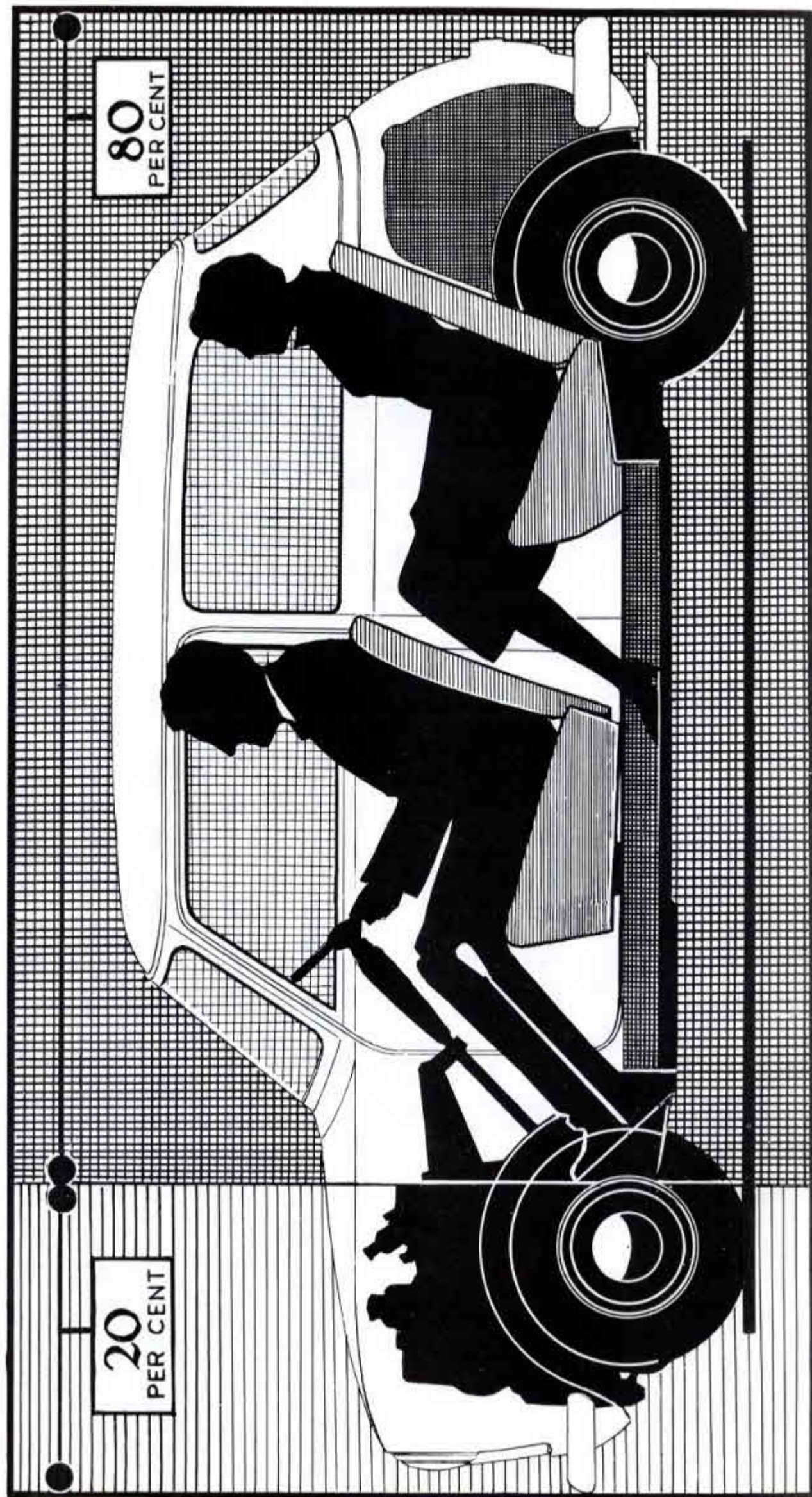
The cut away "Seven" on the Austin Stand shows that 80% of the car's length can be used to carry people or baggage.
